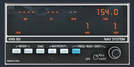
4. When our desired radial is set, press the "DATA" push button once again to enter our desired distance offset of 12.3 nm. Again, should your desired distance include a decimal component, the inner rotary knob can be pulled and rotated for decimal entry.
