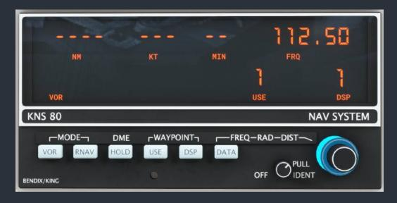
3. Once our desired frequency has been set we will use the "DATA" push button to page through the three required pieces of data in this data channel in the order "FREQ-RAD-DST". Press the "DATA" button once, and then enter the radial 154.0, again with the dual concentric rotary knobs. Should your desired radial include a decimal component, the inner rotary knob can be pulled and rotated for decimal entry.
